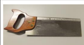
Tenon saw - cuts straight lines in wood
